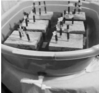
Figure 2. The reinforced concrete samples semi-submerged in the Caspian sea water
