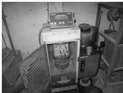
Figure 3. Measuring device of concrete compressive strength during testing of samples after 150 days of exposure to Caspian sea water
