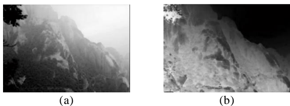
Figure 4. Dark channels: (a) dark channel of the input image and (b) dark channel of the inverse image
