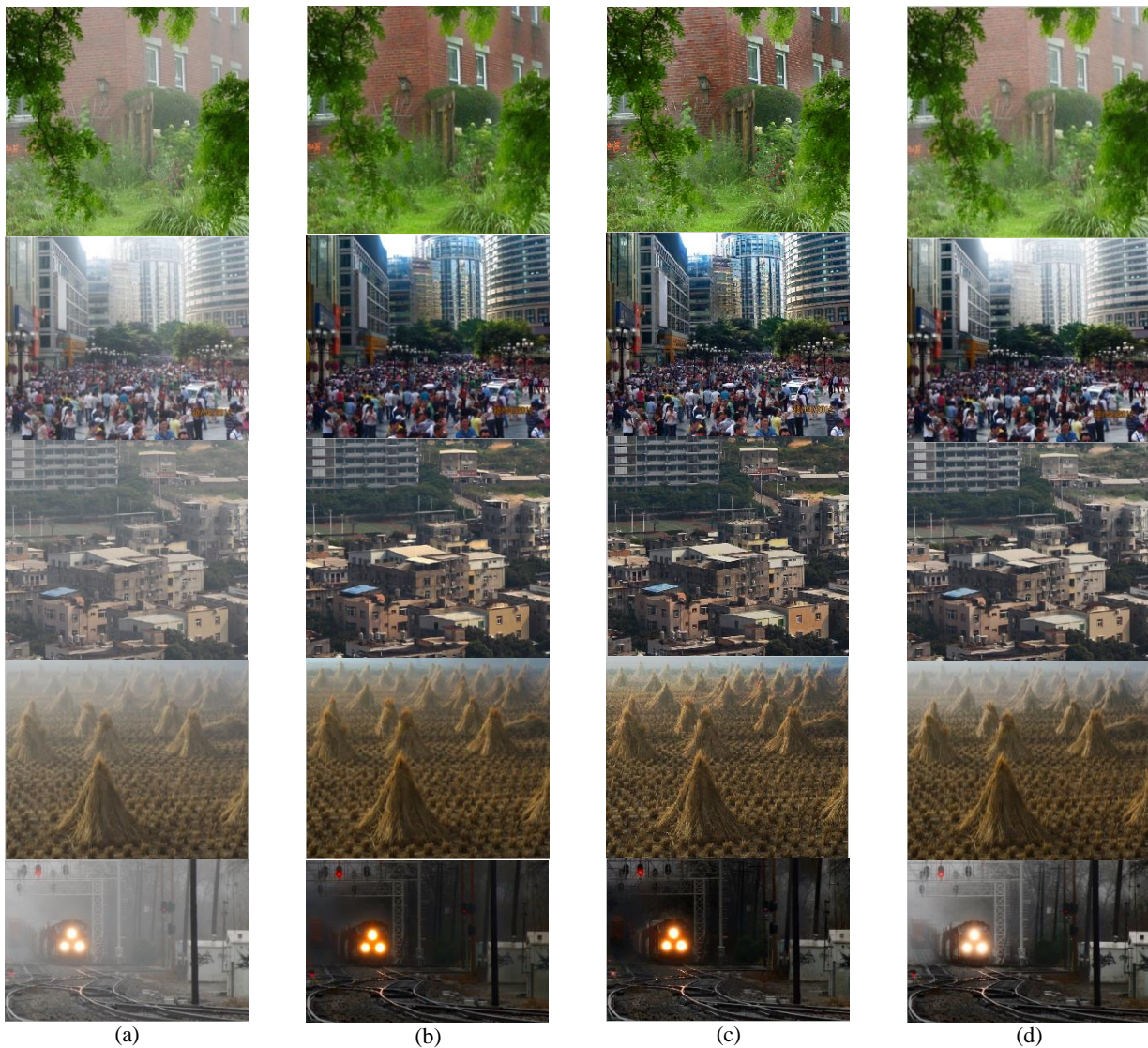
Figure 10. Foggy images and dehazed images with non-sky region: (a) the foggy images, (b) He et al. [9], (c) Jiang et al. [10], and (d) the proposed
