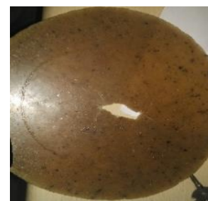
Figure 10. Manufactured Pigmented foil with TiO 2 and BaSO 4 embedded in LDPE matrix
