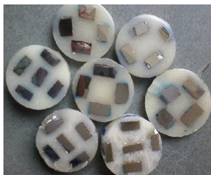
Figure 3. Samples for microstructure examination
