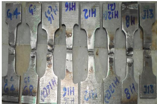
Figure 2. Samples for ultimate tensile strength as per ASTM [17]
