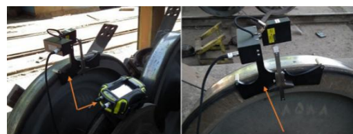
Figure 2. The laser view instrument (indicated by arrows) to measure the wheel profiles
