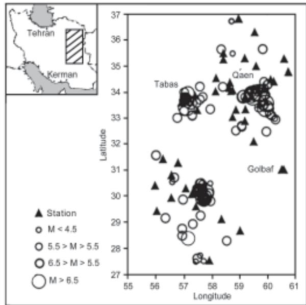
Figure 1. Location of earthquakes and recording stations.
