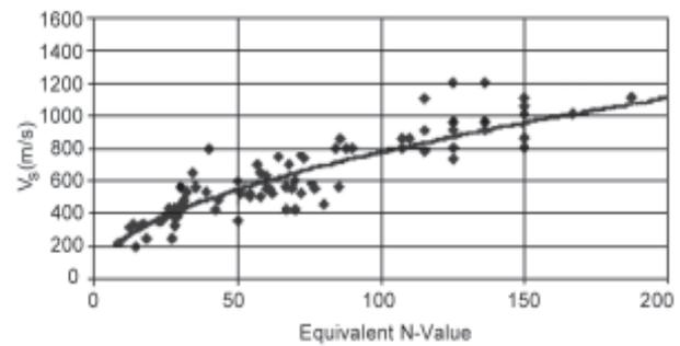
**Figure 3a.** Relation between equivalent SPT value and S-wave velocity for uncohesive material.
