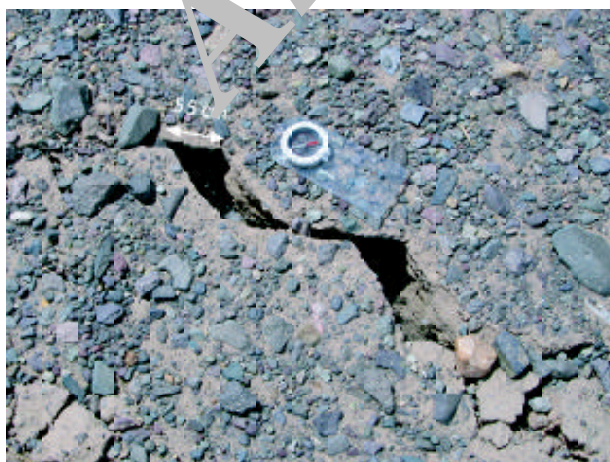
Figure 12. Maximum 5.5 cm lateral displacement measured south of Bam.
