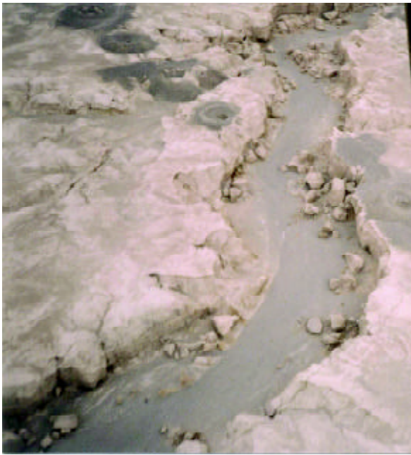
Figure 27. Soil block falls triggered by Bam earthquake at west of Baravat. (The photo has been taken during pilot study by helicopter).
