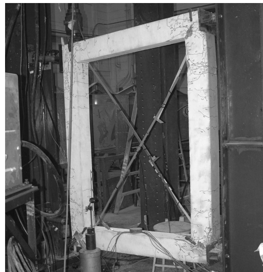
Figure 5. Photo of the moment frame, F1, after the test.
