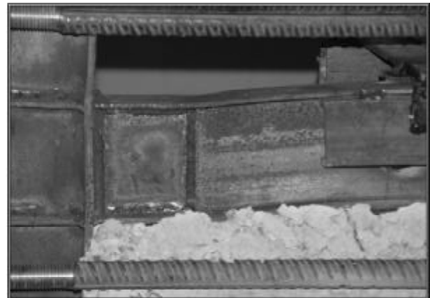
(b) Plastic Hinge in Top Beam
