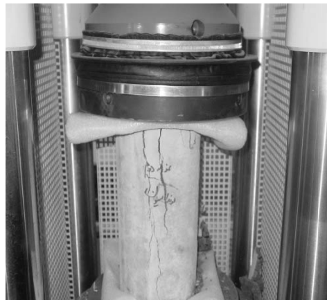
Fig.6 Cylindrical sample under compression test
