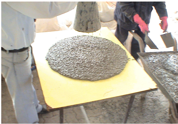
Fig. 2. Slump flow test of SCLWC
