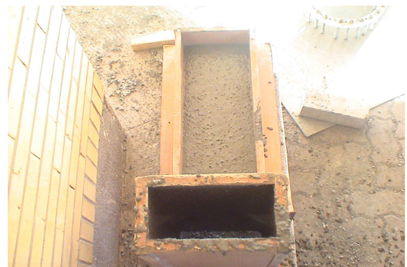
Fig. 5. L-box test of SCLWC
