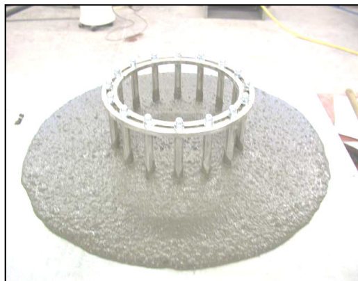
Fig. 3. J-ring test of SCLWC
