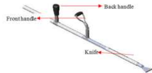
Fig. 6: New design harvesting tool.
