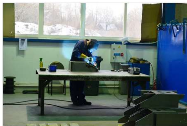
Fig. 2: Welder's workplace, Migatronic equipment (Company A)
