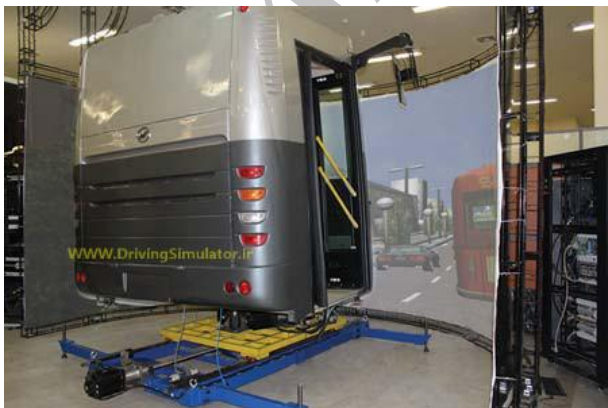
Fig. 1: Driving simulator model AKIA-BI 301
