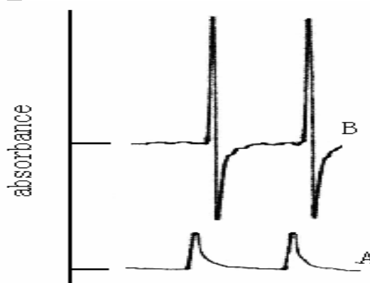
Fig. 3. Absorption signal of conventional (A) and derivative (B) FI-FAAS.
