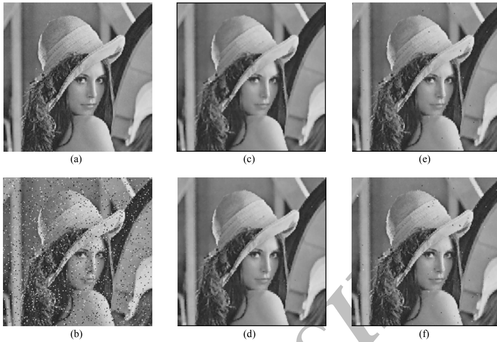
Fig. 4. Achieved results using the test image Lena: (a) original image, (b) noisy image with p_n = 0.1 , (c) output of the median filter, (d) output of the non-adaptive LMA WM filter, (e) output of the adaptive sigmoidal WM filter, (f) output of the genetically optimized WM filter.
