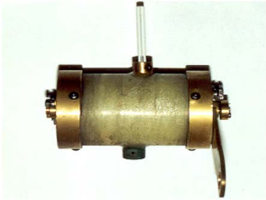
Fig. 1. Photograph of the test fuse: length is 112 mm and inner diameter of the cartridge is 59.5 mm.
