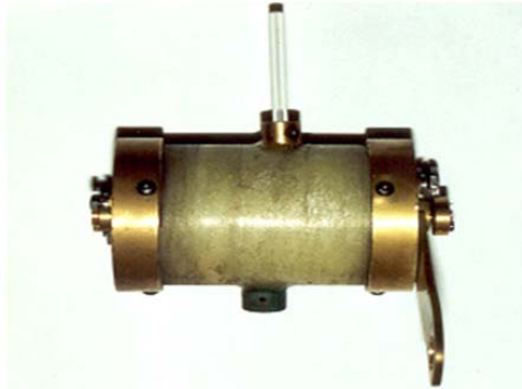
Fig. 2. The short fuse, 112 mm long with inside diameter of 59.5 mm.
