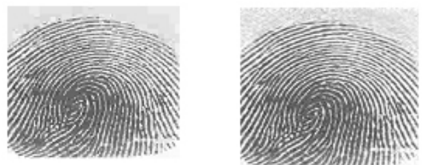
Fig. 17. Fingerprint-B reconstructed using 3 levels of decomposition for bpp=1 by (a) WT SPIHT. (b) CT- SPIHT.
