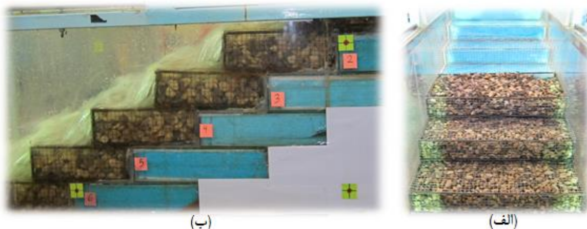
Fig. 3- Installing gabion packages on stepped spillway
