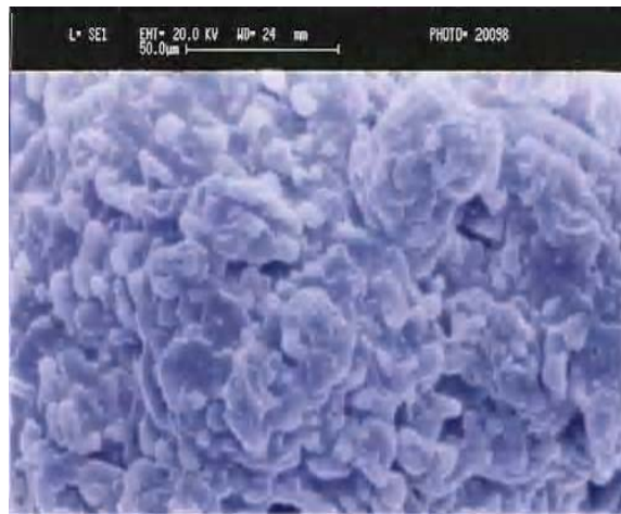
Fig. 5: Scanning electron micrograph of Pb (II) treated SILP showing dense agglomerated, etched cluster type morphology
