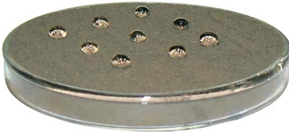
Fig. 1: Determination of water repellency by the molarity ethanol drop method
