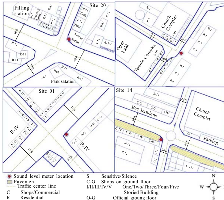
Fig. 1: Typical representative locations showing the road geometry, site plan and noise sampling locations
