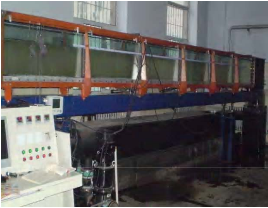
Fig. 3: The test flume line, commercially available 0 # diesel fuel was chosen. The viscosity is 8.5-9.5 mm/s at 5 °C, density is 0.835 g/cm, and freezing point is -2C
