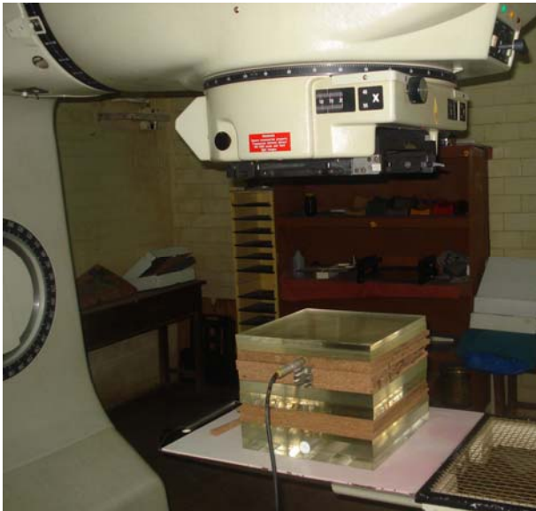
Figure 1. Experimental setup of PMMA and cork slab phantom and the ion chamber inserted in the cork slab to measure the lung dose
