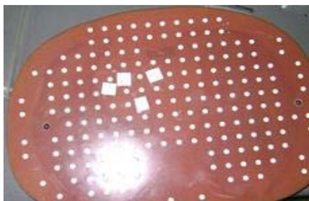
Figure 9. Location TLDs in heart region for practical dosimetry
