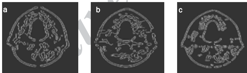
Figure 4. The optimized “Canny” edge detection algorithm response applied for CT image difference slices for (a) 1 pixel horizontal and (b) 1 pixel vertical image displacement and (c) 1 degree image rotation around the image centre.
