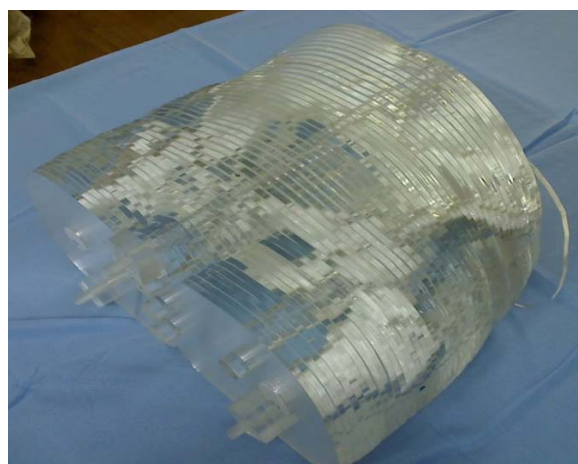
Figure 2. Heterogenic anthropomorphic pelvic phantom and its Inserts.
