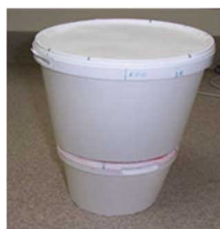
Figure 2. Two can phantoms with lid kept one over the other simulate the regions above and below the knee in terms of variations in thickness, as well as tapering effect. The bottom side of the top can and top side of the bottom can filled with 8 mm thickness of dental wax, to provide smooth surface as well as no air gap for keeping a film in between. Water is filled in the two cans to provide scattering conditions similar to leg.
