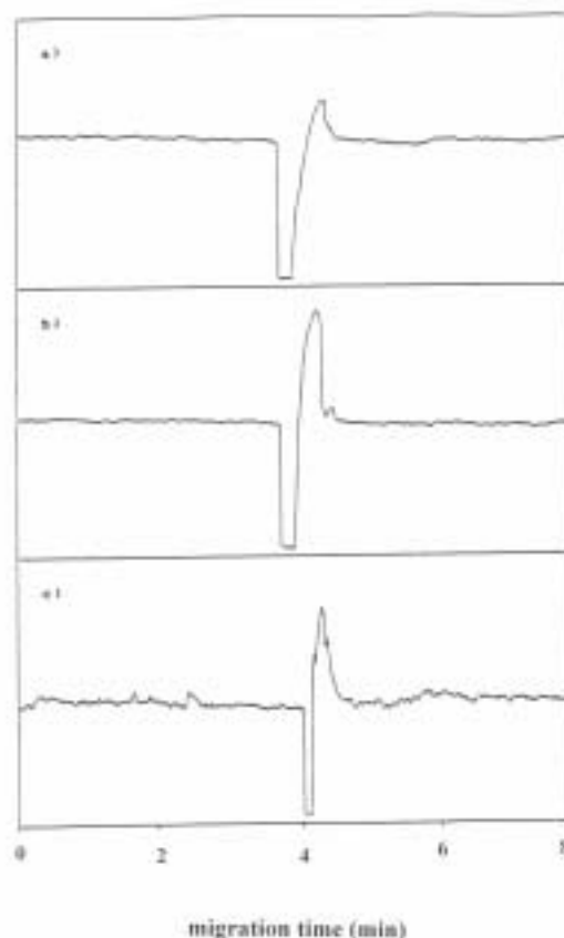
Figure 3. Electropherograms of supernatants of serum samples deproteinised with acetonitrile 60%. (a) Blank serum (b) serum spiked with methimazole (0.02 mg/ml) using a CZE method with the conditions as described in Figure 2 and (c) the same as (b) but using a MEKC method (50mM SDS was added to the CZE buffer).
