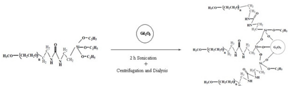
Figure 3. Reaction scheme showing the functionalization strategy when capping \text{Gd}_2\text{O}_3 Nanoparticles with m-PEG-silane. This reaction shows mPEG-silane coated with SPGO by silane linker molecule.
