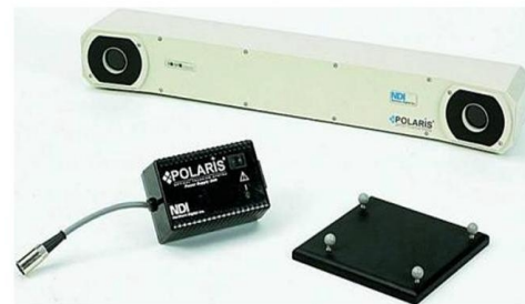
Figure 1: The POLARIS system uses four infrared-reflective spheres placed in a precisely known geometry.
