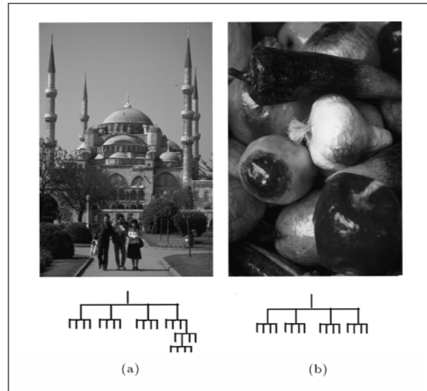
Figure 5. A quad-tree representation of two images. (a) An unbalanced quad tree with high depth with 29 nodes; (b) A balanced quad tree with low depth with 21 nodes.
