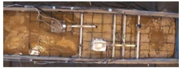
Figure 17. Ground surface after liquefaction and lateral spreading in test no. 2. Note the development of tension cracks at upslope and development of sand boils at different places [85].
