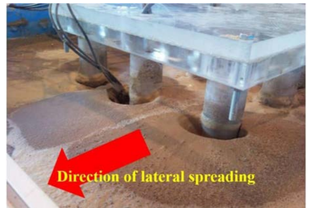
Figure 19. Gap formation at the downslope side of the piles in the downslope row of 3x3 pile group and heave of soil at the upstream side of the piles in test no. 3 [83].
