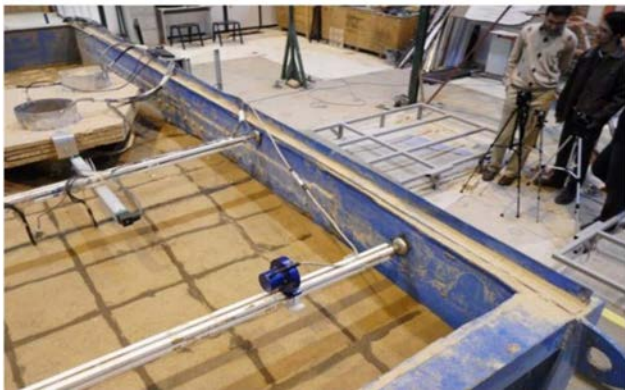
Figure 20. Lateral spreading and associated settlement at upslope side of the ground in test no. 4 [87].
