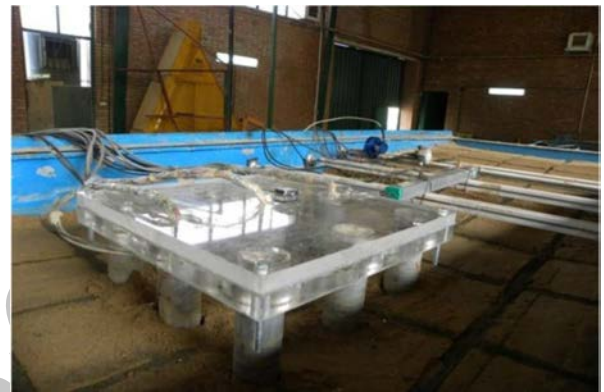
Figure 18. A general view of the 3x3 pile group in the 3rd test.
