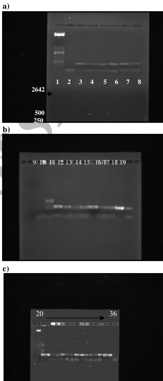
Figure 2. a, b, and c: Agarose gel electrophoresis of PCR products of the M. tuberculosis rpoB gene. Lanes 1 and 20 are ladder 50. Lanes 2, 9 and 36 are negative control. Lanes 3 to 8, 10 to 19, and 22 to 36 show PCR products of the M. tuberculosis rpoB gene (resistance and sensitive strains). Lane 10 show two bands, lane 21 shows PCR products of the BCG extracted DNA and lane 22 shows PCR products of rpoB gene of the H 37 Rv extracted DNA.
