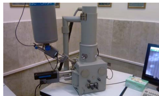
Fig 5. Electronic microscope used for the project fractography
