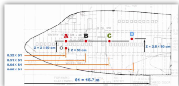
Figure 17. Illustration of selected point for fatigue crack growth analysis
