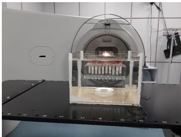
Fig. 3. Irradiation set-up using compact external beam radiotherapy machine
