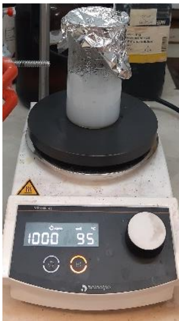
Fig.1. Nanoparticles precipitate was mixed with 100 ml of deionized water and placed at 100 °C for 5 and a half hours
