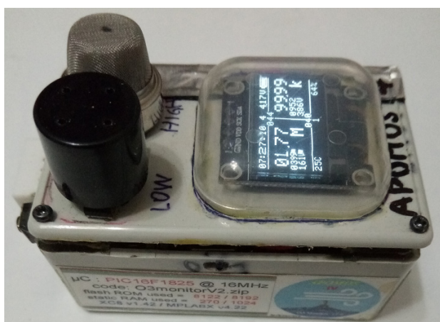
Figure 3. The APOMOS equipped with MQ131 detectors for low and high concentrations, and the DHT22 sensor for measuring temperature and humidity.
