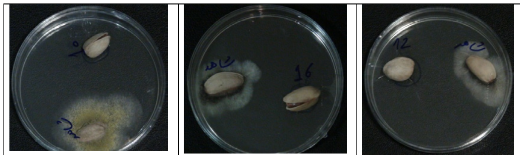
Fig. 6. Antimicrobial activity of coated PLA nano-composites containing ZnO 1%, 3% and 5% (a, b and d) and uncoated pistachios against Aspergillus parasiticus (PTCC5018)
