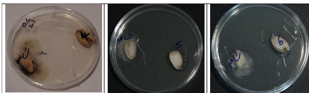
Fig. 5. Antimicrobial activity of coated PLA nano-composites containing ZnO 1%, 3% and 5% (a, b and d) and uncoated pistachios against Aspergillus parasiticus (PTCC 5286)
