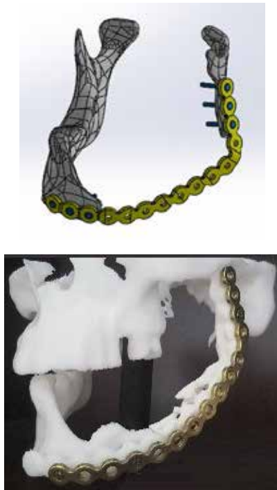
Fig. 2. A 3-D model of the patient's artificial mandible made by the additive manufacturing technique.
