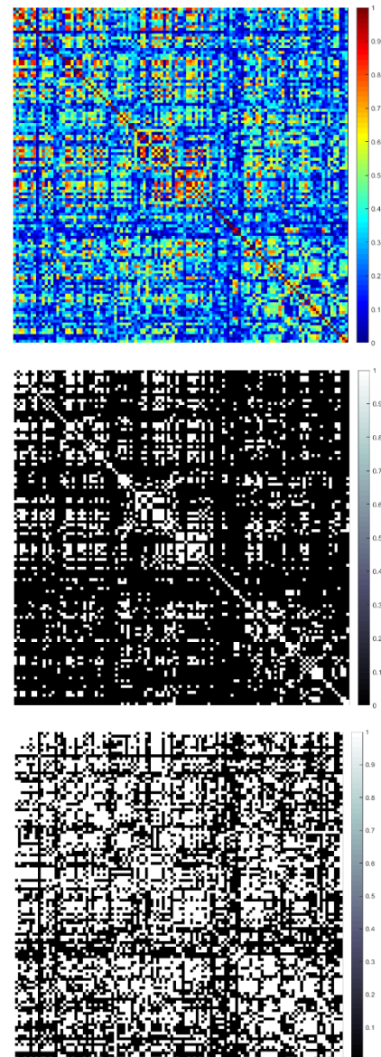
Figure 2. A functional connectivity matrix. A weighted matrix (up). A binary matrix which is sparsified by threshold 0.5 (Middle) and a binary matrix which is sparse by density 50% (bottom)
