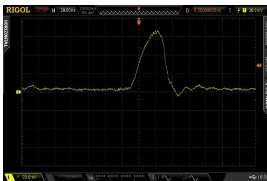
Figure 3. Optical pulse that is generated by high power LED mounted on driver board
