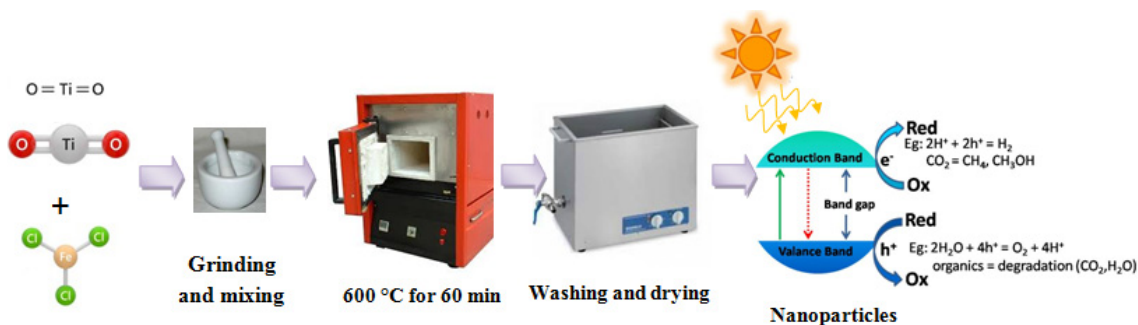
Fig. 1. The schematic of the preparation process of TiO 2 nanoparticles
