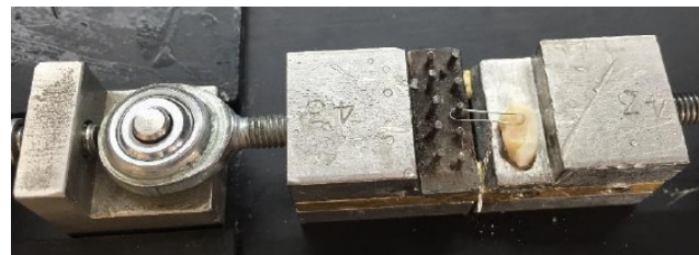
Fig. 2- Shear bond test by universal testing machine
