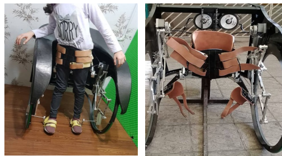
Figure 2. The designed "gait enhancer" device
