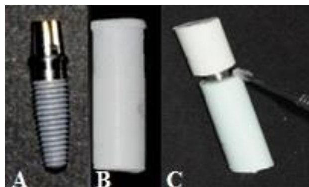
Fig. 3: Samples mounted in putty for measuring microleakage, (A) implant and abutment, (B) implant and abutment covered with putty (negative control), (C) applying adhesive with a brush
