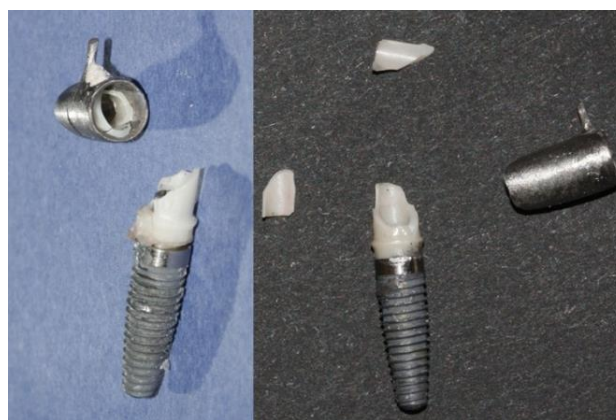
Fig. 4: Two broken ceramic samples during cyclic loading process, the fractures were on the walls not connections
