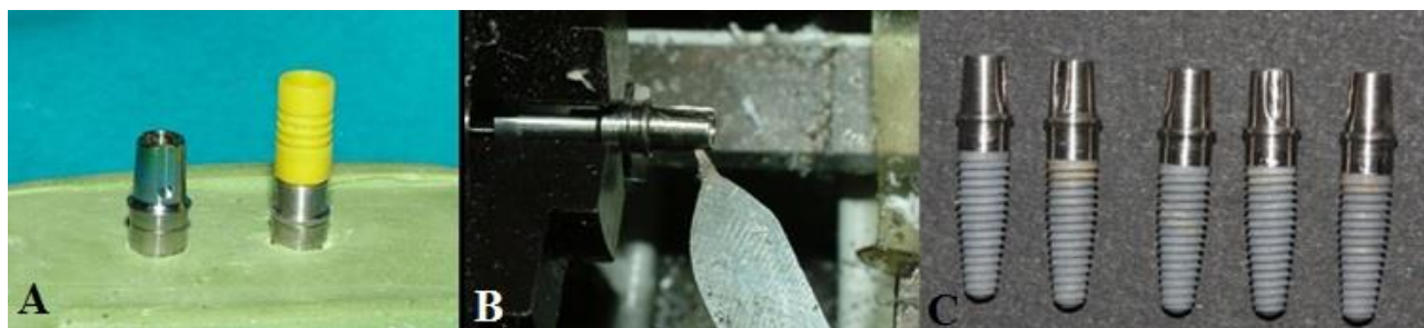
Fig. 2: Fabrication process of GoldAdapt samples, (A) wax up, (B) milling procedure, (C) GoldAdapt samples
