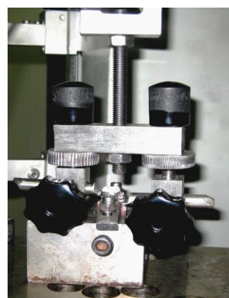
Fig. 2: Customized band removal device used to simulate clinical load for measurement of retentive strength
