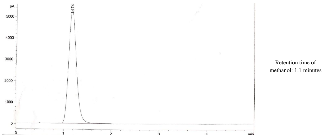
Figure 2. The chromatogram of the analyzed alcoholic beverages containing methanol
