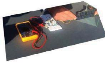
PV cell on the southern vertical wall with vertical mirror on eastern side
